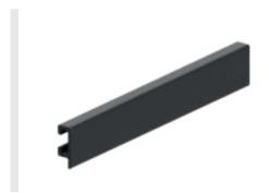
Side guides are used for reliably guiding the product on roller conveyors and belt conveyors, as well as on the corresponding components. We offer the side guides in an aluminum and a polymer version. In particular, because of the flexible material, the guides can be adjusted to the material flow in curves, as well as when merging and diverting.
